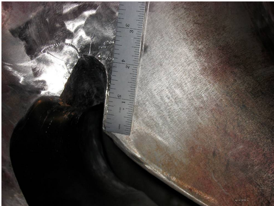
Photo 1: Crack location in rib between buckets 5&6
