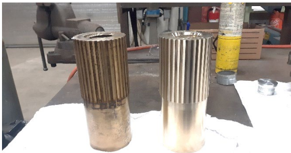
Figure 3. New SF25 stem nut machined in-house (Right) Original SF25 stem nut with stripped internal threads (Left)
