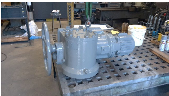
Figure 5. Fully assembled and refurbished limiter torque operator ready for another 65 years of service at SF25
