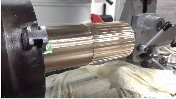
Figure 1. Milling complete on new SF25 stem nut splines
