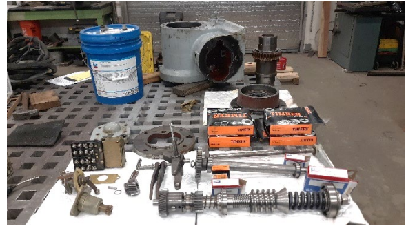
Figure 2. New seals, bearings, and cleaned internals are ready for assembly for the SF25 operator
